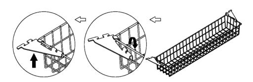
Attach brackets to hang rail at 45° angle as shown in photo below
